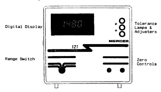
The digital version uses a 3.5 digit display. Metric ranges cover 1999 to 199.9 microns. Inch ranges cover 0.1999 to 0.01999 inch. Digital resolution is 0.025% of scale. Inch and Metric and Metric only versions are available.
